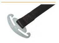
53-1525 Zink plated spreader bar made of 2,5 mm steel. 33 mm and 27 mm web slots. Total width 89 mm.
